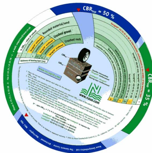
Figure 3. Design disc for bearing layer reinforcement in traffic areas using welded Secugrid® geogrids
