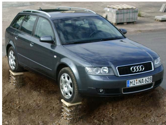
Figure 1. Geogrid reinforced gravel columns carrying a car
